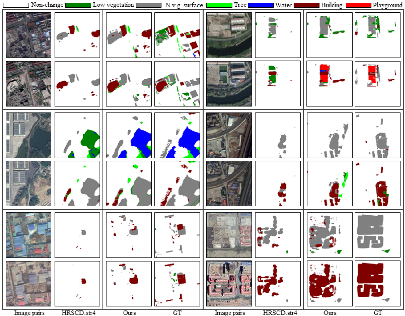
Fig. 7. Visual results of comparison with state-of-the-art method when the encoder is built on residual blocks. We mask the semantic prediction maps with change maps to represent the prediction of change type in each position, where our proposed ASN can better identify land-cover classes and alleviate false identifications of non-change pixels.
